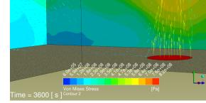
Thermal beam deformation due to fire
