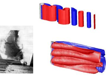
Shedding from chimney with and without helical strakes applied
