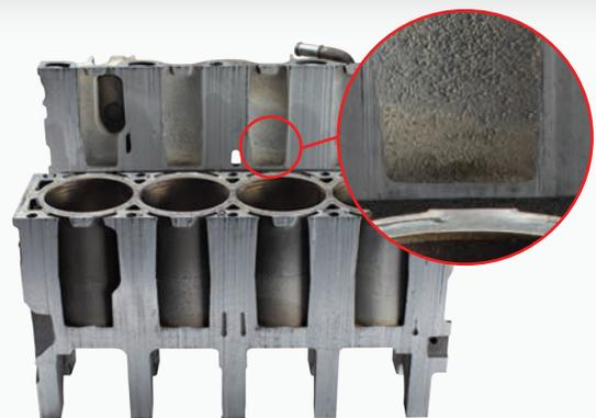
**Engine blocks have cooling passages so heat can be pulled away from the pistons & cylinders**
