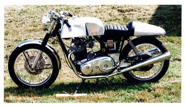
I made rear set controls from pictures I saw in "Classic Bike". They are 4130 chrome-moly tubing and chrome plated. Rear brake set uses stock brake light switch. I made a shorter cable to replace
