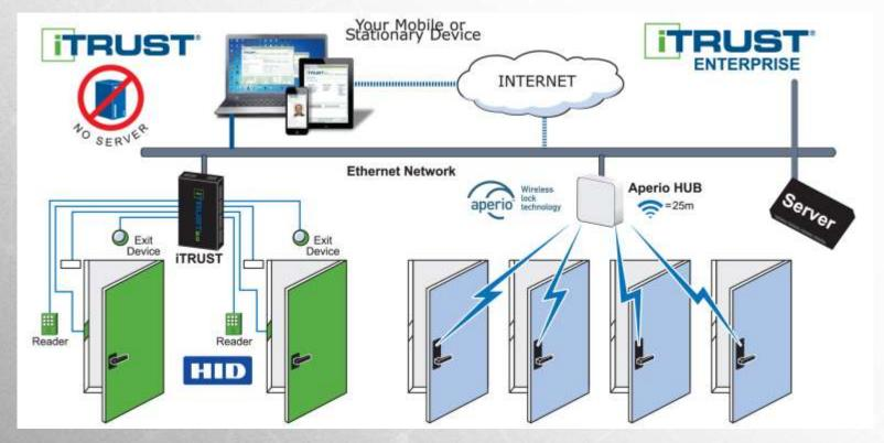
iTRUST access control technology which may be implemented by itself or in conjunction with most access control systems. Oredentials are assigned at the time of card enrollment ensuring authorized access control is in place for designated storage lockers and points of entry.
