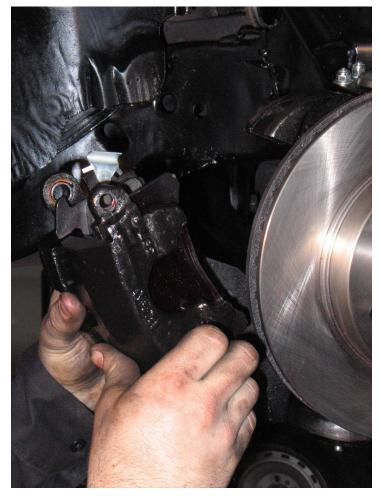
The disc brake conversion is completed by bolting the single-piston calipers to the drop spindles.
