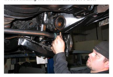
The rivets that hold the factory sway bar mounts in place are blasted off with an air chisel. Then, new frame mounts and poly bushings are greased and installed along with the Hellwig bar.
