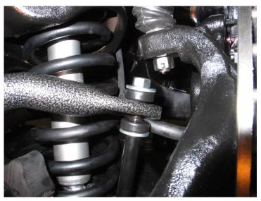
New end links require enlarging the factory mounting holes in the lower control arm but otherwise the bar attaches in the same manner as the old one.
