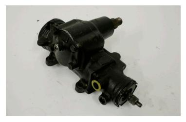
Joe's Elco had enough slop in the factory steering box that no adjustment of the set screw would cure it. We replaced the old box with a quick-ratio unit, which shortened the lock-to-lock turns of the steering wheel and improved steering input.
