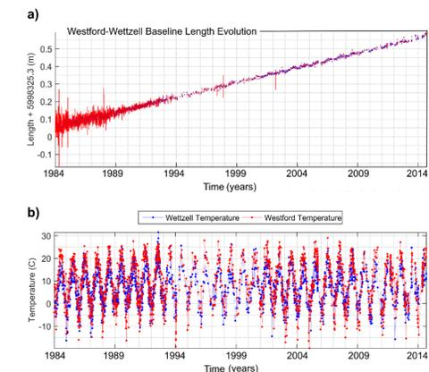
Fig. 9 (a) The unequally spaced VLBI baseline length evolution since January 1984 with error bars (red) (b) Unequally spaced and equally weighted temperature series at stations Westford (red) and Wetzell (blue) since January 1984. (c) and (d) The LSCWS of the residual VLBI series (baseline length and temperature) in Westford and Wetzell, respectively with their stochastic surfaces at 99% confidence level (gray) and phase differences (white arrows).
