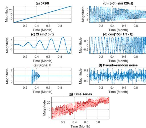
Fig. 4 The unequally spaced time series and its constituents. (a)-(f) different constituents and (g) the time series (the sum of the constituents).
