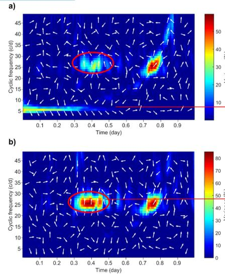
Fig. 7 (a) LSCWS of the time series (b) LSCWS of the residual time series after removing (suppressing) the peaks at 5c/d. The arrows on the spectrogram show the phase differences.
