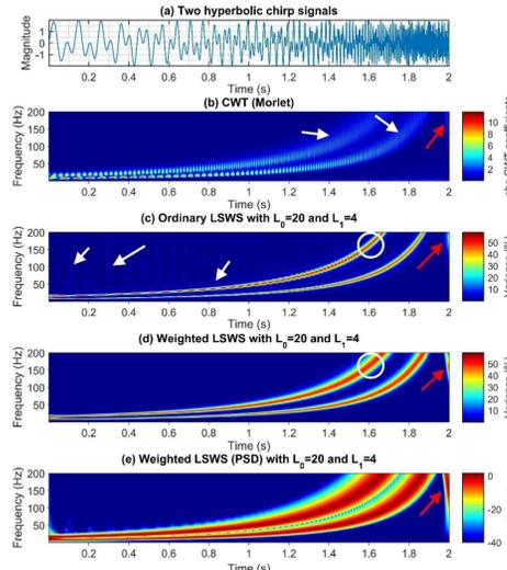
Fig. 3 Two hyperbolic chirp signals and their analyses.
