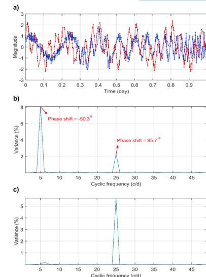
Fig. 6 (a) Two unequally spaced series (b) Least-squares cross spectrum (LSCS) of the two time series (c) LSCS of the two residual time series after suppressing the peak at 5 c/d
