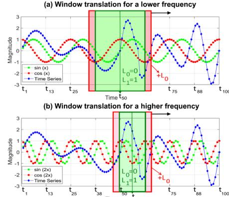
Fig. 2 Window translation of an equally spaced time series (blue) for (a) sin(x) and cos(x) and (b) sin(2x) and cos(2x).
