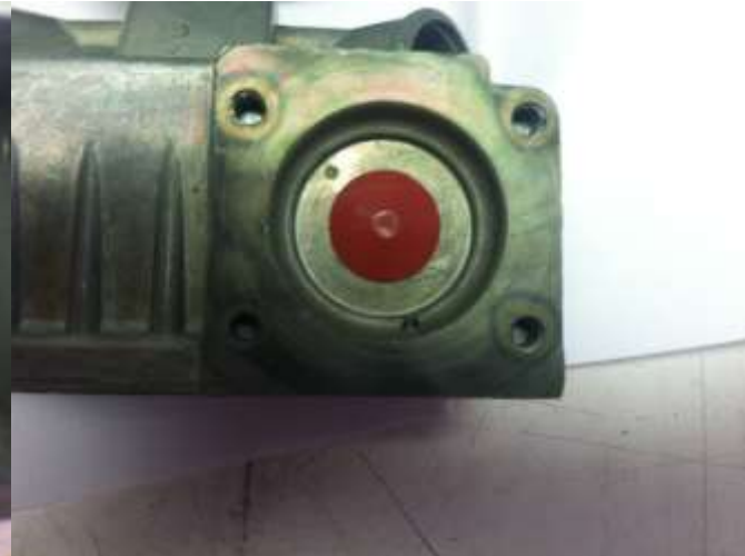
Accelerator Pump Assembly Part # 34R-12684B
