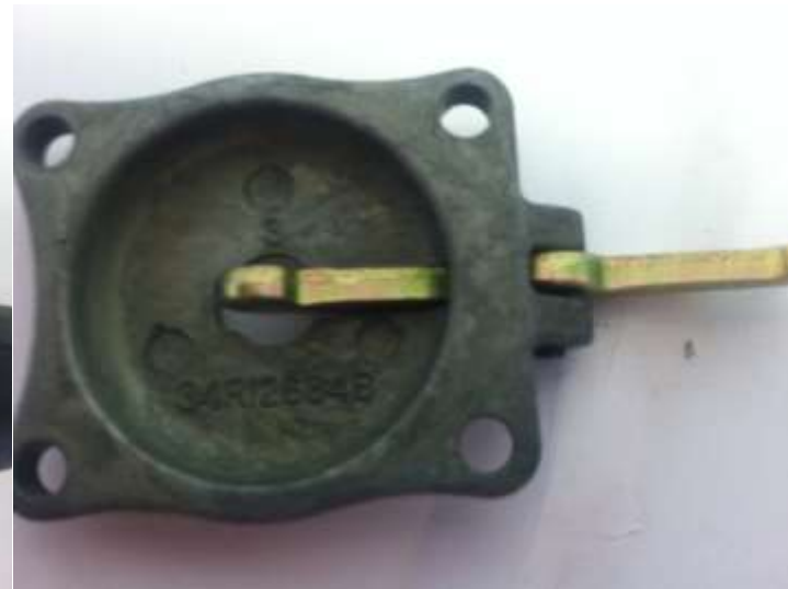
Accelerator Pump Assembly Part # 34R-12684B
