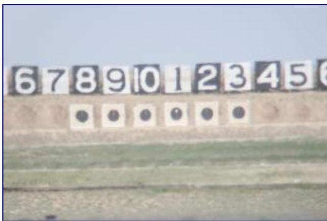
Through the spotting scope, the targets are distorted by mirage, but the spotting disks are visible on several of the targets.
