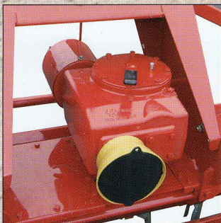
3-speed leverchange gearbox with rear PTO.
