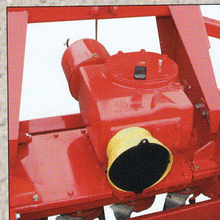
3-speed leverchange gearbox with rear PTO.
