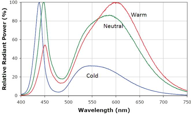
Fig. 1: Relative radiant optical power of Cree Xlamp XR-C LEDs (Graph image is the property of, and is used by permission of Cree, Inc).
