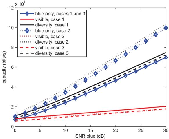
Fig. 3: Channel capacity for three receivers versus received SNR blue.
