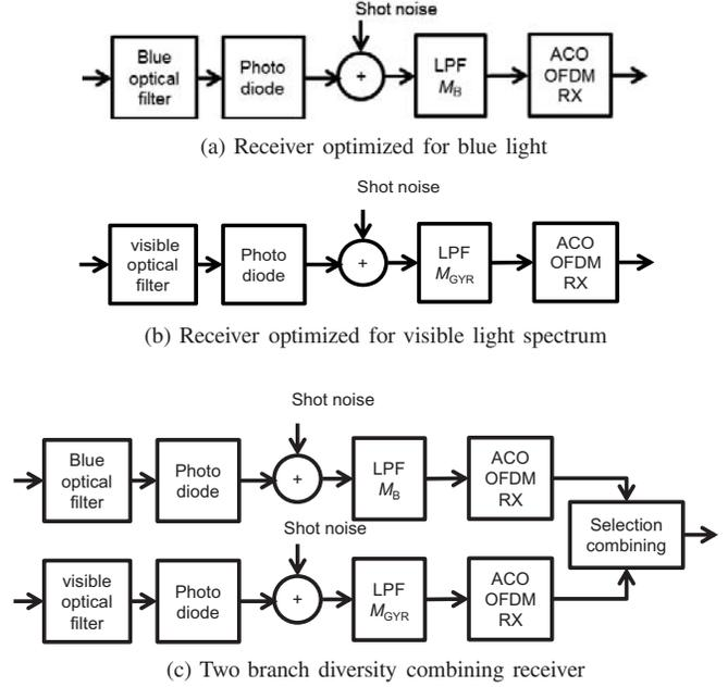
Fig. 2: Block diagrams of the three receivers
