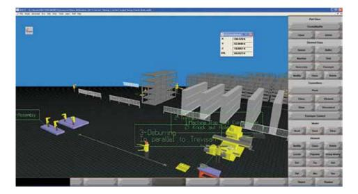
What was the result? We implemented the layout as modeled. Impressively, the travel distance from picking raw material to final test was reduced by 90%! Co-location of the equipment in, along with dedication to, the line drove most of the improvement. Re-locating raw material stores also helped significantly in terms of time and distance. Some process changes, mostly in machining, helped also. The end results included a 22% increase in PVA (production value added) ratio.
