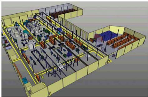
As in the first project, everything builds up from individual models into assemblies. On the next page, you can see the actual product components and the assembly conveyor line, all of which add up into the process line including test rig and paint booth. All the process lines and other equipment, like NC (numerically controlled) machines, add up to the entire factory
