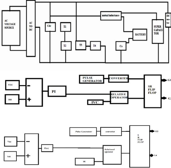
Fig.4: Hybrid energy storage system applied to electric vehicles in PI model and power command
