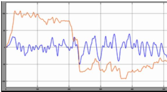
Fig.14: Power of the super-capacitor and Li-ion battery of proposed system
