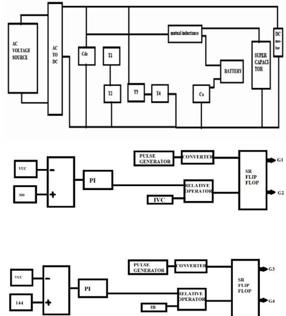
Fig.3: Hybrid energy storage system applied to electric vehicles in PI model
