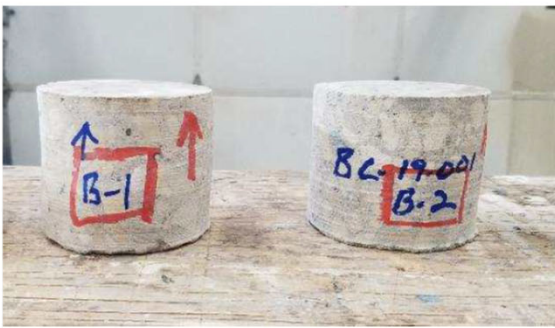
Figure 3 - Roofing concrete cores with MVRA, samples B-1 and B-2.
