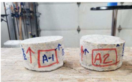
Figure 2 - Roofing concrete cores with MVRA, samples A-1 and A-2.
