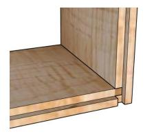
Before assembly, rabbet the back edges of the case sides to receive the cabinet back. Width of the rabbet is half the thickness of your material. Depth is slightly more than the thickness of the back.
