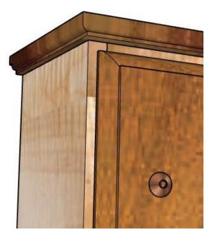
The top overhangs the sides by  $\frac{1}{2}$ ", and the front by  $\frac{3}{4}$ ".
