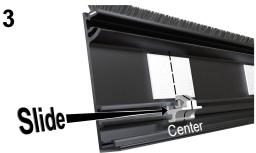
Slide fascia clips into groove and center each clip in middle of each velcro as shown. Ensure clips are aligned to fascia brackets prior to installation.
