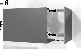
For outside mount fascias, insert tabs of endcap into retaining features on fascia.
