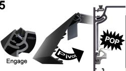
Install fascia by engaging fascia tongue into bracket groove, then pivoting fascia toward bracket until you hear both clips "POP!"
