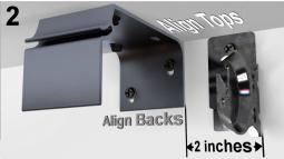
Mount fascia brackets two (2) inches inward from shade brackets' far edge, and so that fascia and shade brackets are aligned at both top and back. Use two (2) screws in jamb or wall, opposite each other as shown.\*
