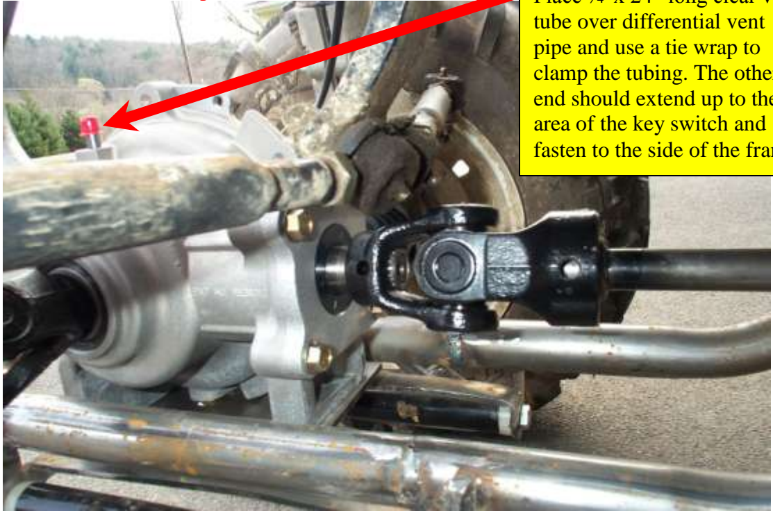
Differential installed (picture)
