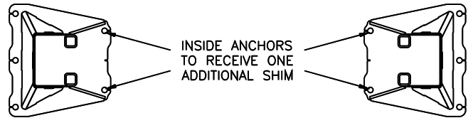
Fig 14 – Front Column Shimming
