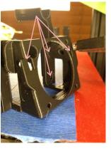
2. Insert (4) 3mm nuts 3. Test fit the screws in in the nut capture slots. the nuts to make sure they are centered.
