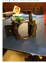
4. Remove the old mount and detatch the stock fans. Lay them to the back. Cut off a couple zip ties from the cable Slide the base to the right and to the back plate. if you need to lengthen wires.
