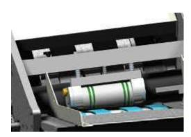
Indexing feed drum quickly rotates without the use of tools or technical adjustment
