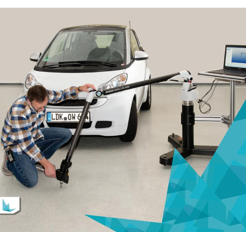
ROMER GridLOK is an expanded measurement solution that allows the accuracy and convenience of the ROMER Absolute Arm to be applied to the inspection and measurement of larger parts and systems.
