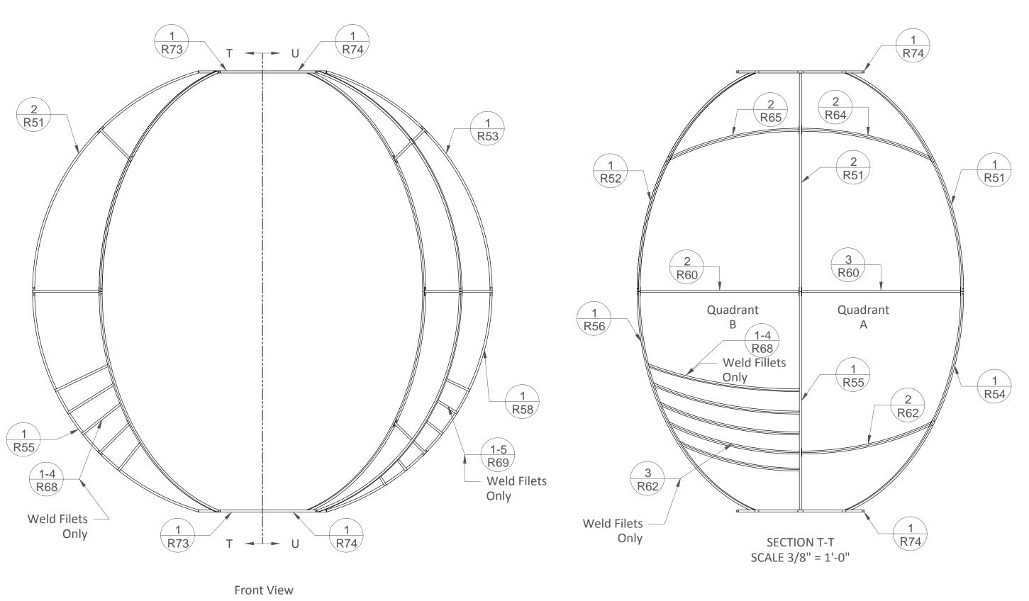
Globe Assembly - Scale:  $\frac{3}{8}$ " = 1'-0" R75 Build 1 from component parts. Bolt with  $\frac{1}{4}$ " Hex Head bolts or weld as indicated.
