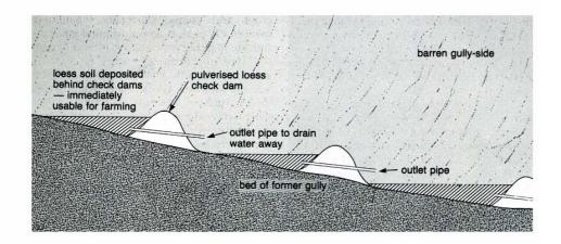
Constructing **check dams** using compressed loess to a height of 6m across gullies. These dams trap silt in stream runoff and allow the water to be drained through pipes.
