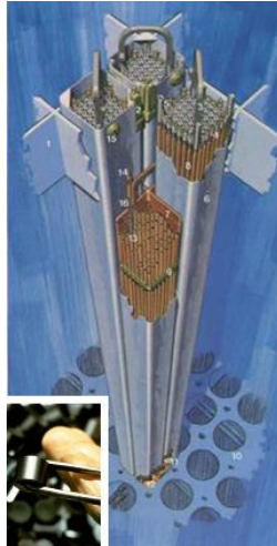
Figure 6: BWR Fuel Rod Assembly and Fuel Pellets (NRC)
