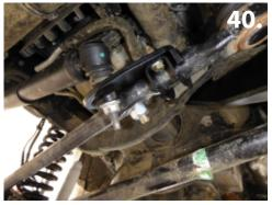
50. Reconnect the steering shock on to the drag link using the factory hardware. Torque to factory specs. (pic 40)
