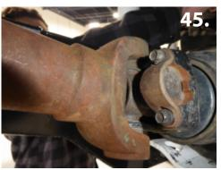
56. Reconnect front drive line using the factory u-joint caps and bolts. Be sure to loctite the bolts when reinstalling. Torque to factory specs. (pic 45)
