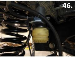
57. If you have not already, you can now install the factory bump stop in to the factory mount and spacer. Be sure to connect the front axle breather hose and vacuum line to the new vacuum line bracket that was installed between the bump stop mount and bump stop spacer on the driver side. (pic 46)
