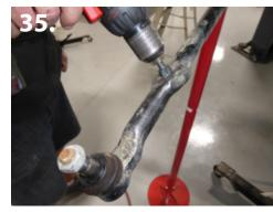
43. Loosen drag link clamp using 15mm and safety retainer using 13mm. (pic 34) 44. Now rotate drag link so that the end link faces up.
