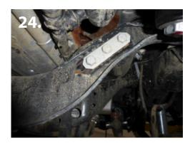
31. Install new track bar drop bracket using all the factory hardware. (pic 23)
