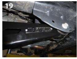
24. Install new McGaughy's radius arms on driver side and passenger side. Use the provided cam bolts and washers for the lower mounts on the axle. (pic 17-18) Be sure to use the cam washers on both sides of each radius arm.
