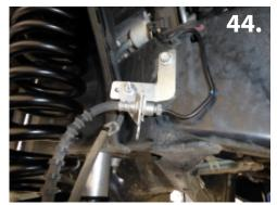
55. On passenger side, install new brake line bracket using the factory hardware. Reposition brakeline as shown and connect the factory brake line bracket on to new brake line bracket using provided hardware. (pic 44) Make sure the brake line is not rubbing anywhere that could wear a hole in the line.
