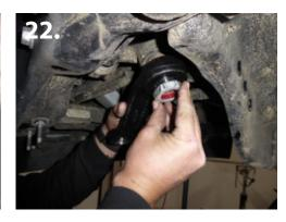
28. Install the provided drag link flip collar in to new provided pitman arms. (pic 20-21)
