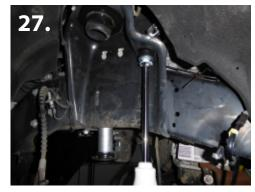
34. Install new bump stop drop spacers. Use the provided 15mm bolt to install through the factory mount and spacer up in to the factory location on the frame. On the driver side, you will sandwich the vacuum line bracket betwen the mount and spacer. (pic 25-16)
