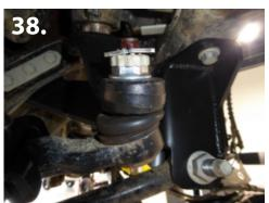
48. Reconnect the drag link to the pitman arm using the provided 14mm flange nut. **DO NOT USE THE FACTORY NUT.** Torque to factory specs. Next install the factory crown retainer and cotter pin, to secure the flange nut. (pic 38)
