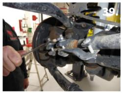
49. Tighten drag link clamp and safety retainer on drag link. **Be sure to align the vehicle before driving.** (pic 39)
