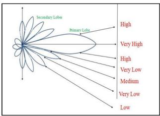
Fig.1: Radiation Pattern of Cell Tower Antenna
