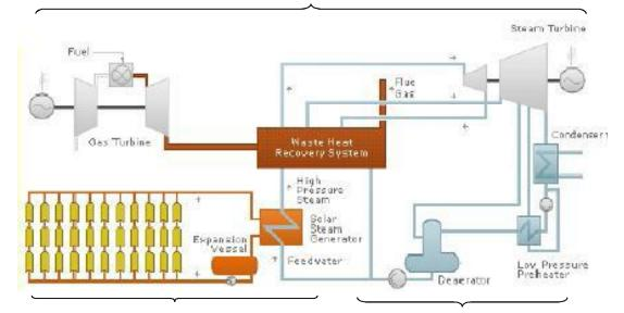
Solar field Solar Resource: 2,060 kWh/m2/yr Output temperature = 393°C
