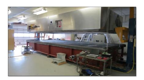
Large-scale calibrated hot box (8 ft. x 24 ft. specimens)
