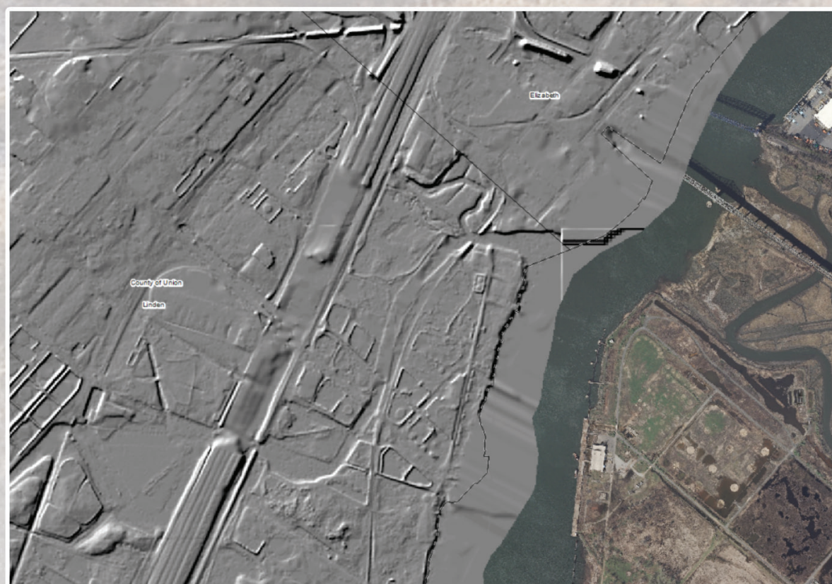
The statewide 10-foot DEM was created from various LiDAR datasets flown at different times.
