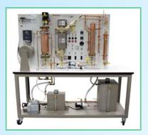
The Hampden **Model H-ETS-1A** Ethanol Production Process System is designed to facilitate the instruction of students on the process required to produce ethanol for experimental purposes. Ethanol is a very promising fuel alternative to oil since sources are widely available and ethanol is clean-burning. The student will be able to observe and control the process of producing
