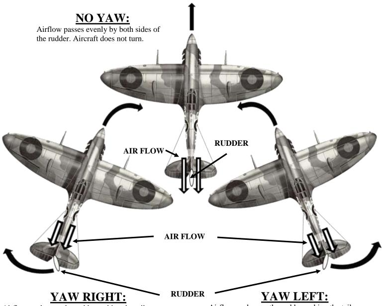
Airflow pushes on the rudder making the tail move left. When the tail goes left, the nose moves right.
