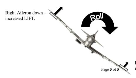
ROLL LEFT: Pilot moves control stick to the left. The right aileron moves down while the left aileron moves up. Lift will be increased over the outer part of the right wing and reduced over the outer part of the left wing. The aircraft will roll to the left.
