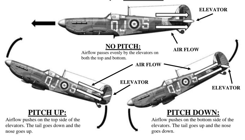
**NO PITCH:** Airflow passes evenly over both the top and bottom of elevators. Aircraft will continue flying straight until the elevators are moved by the pilot.
