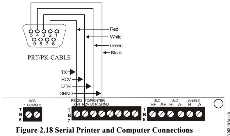
Figure 2.18 Serial Printer and Computer Connections
