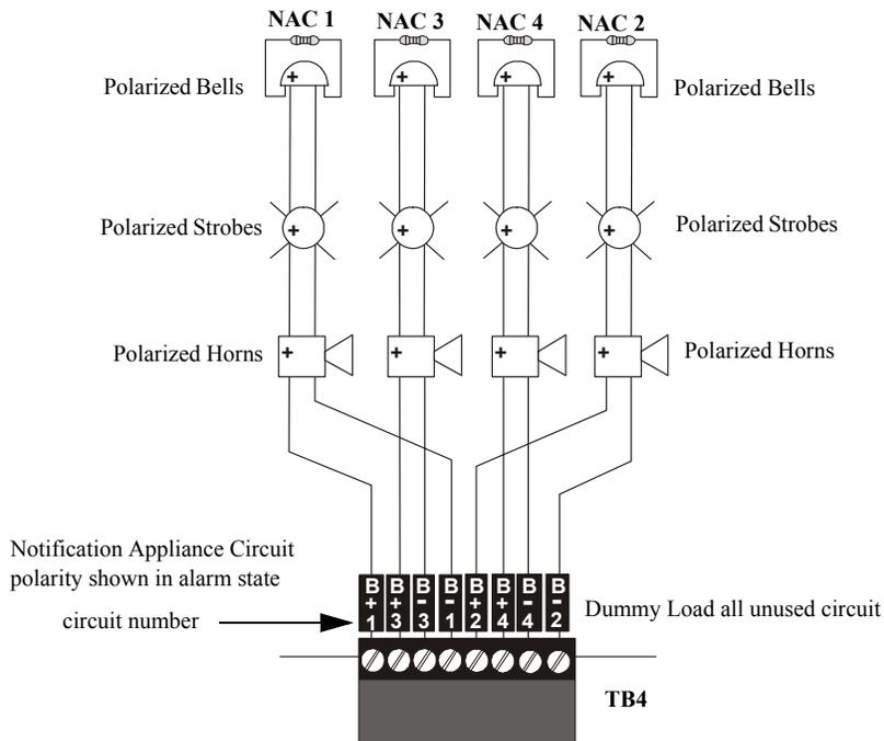
Figure 2.7 NAC Style Y (Class B) Wiring
