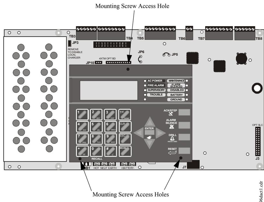
Figure 2.10 Keypad/Display Removal
