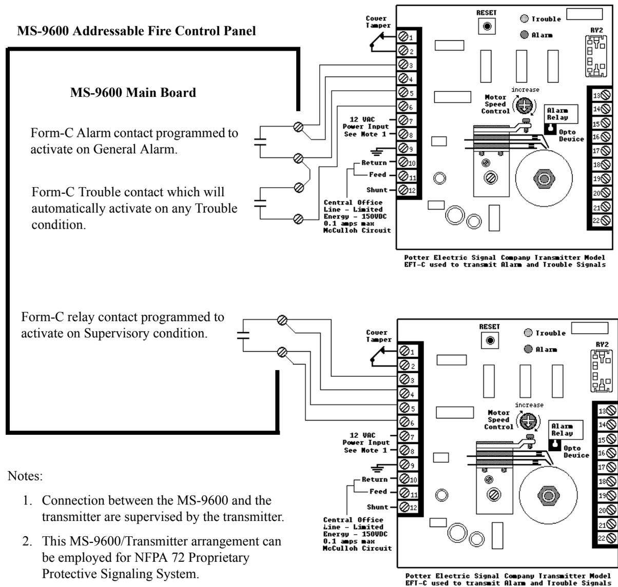
Figure C.6 Proprietary Protective Signaling System
