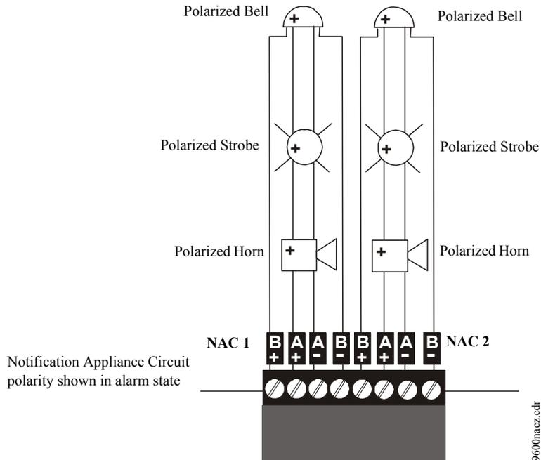
**Figure 2.8 NAC Style Z (Class A) Wiring**
