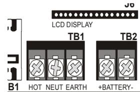
Connect a wire from the grounding stud in the cabinet to a known solid earth ground (refer to Figure 2.1 on page 24). This connection is vital for maintaining the control panel's immunity to unwanted transients generated by lightning and electrostatic discharge. Apply AC power to the panel only after the system is completely installed and visually checked. *Note that AC power must be applied to the panel before installing the battery interconnect cable (refer to the following section).*
