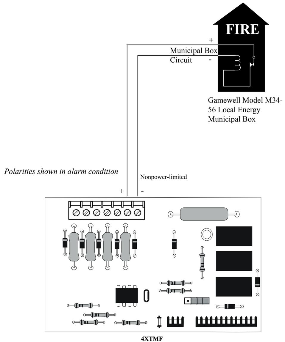
**Figure C.4 Municipal Box Connected to 4XTMF Transmitter Module**
