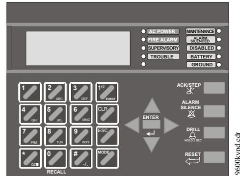
Figure 1.2 Membrane/Display Panel
