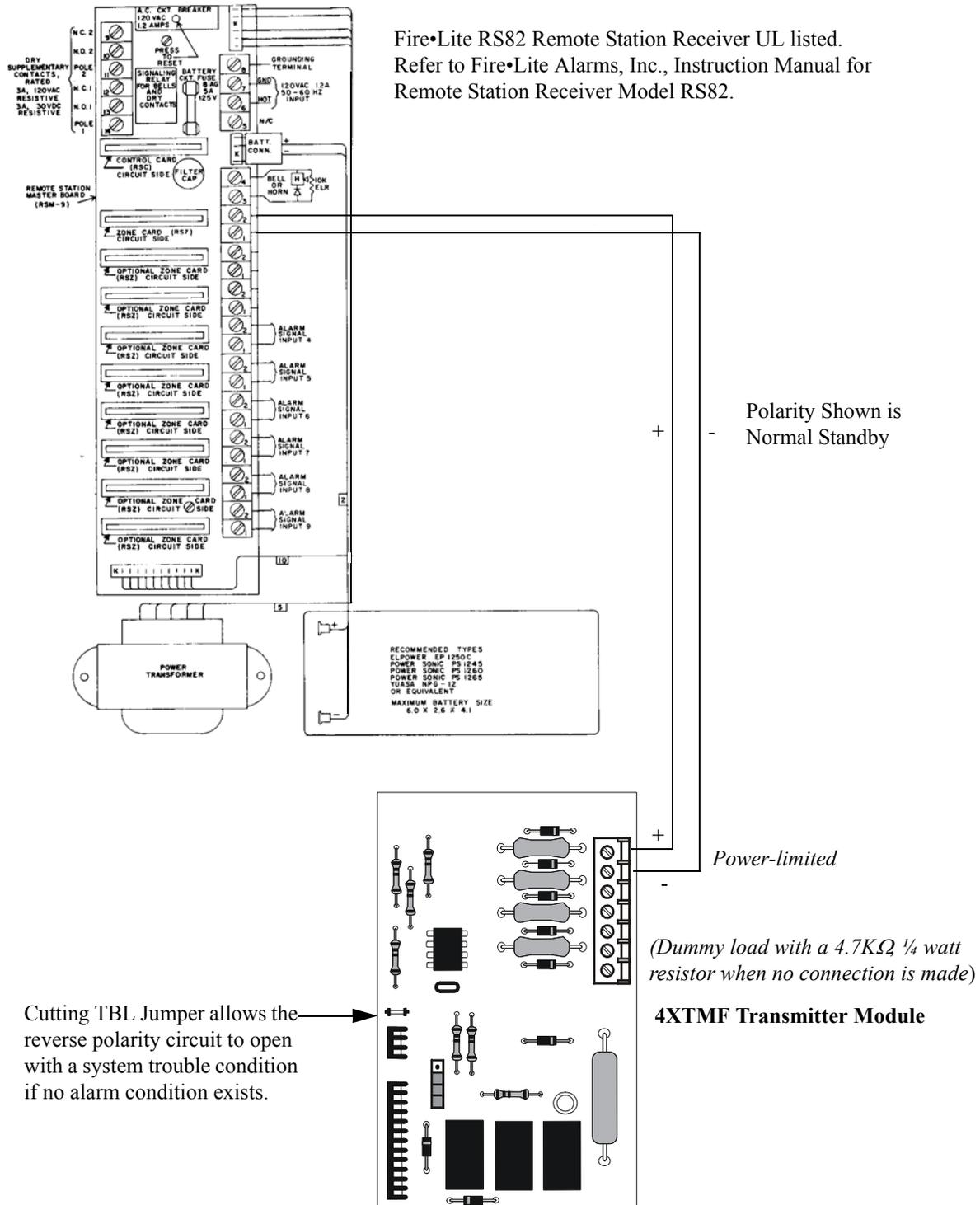
Figure C.5 Remote Station Connection Using 4XTMF Module
