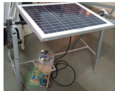
Fig.6 Monitoring and Controlling Circuits for Load Control
