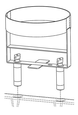
Insert the 5 Gallon Bucket Holder into the chosen location by aligning the anchors with the holes on the bed sides.
