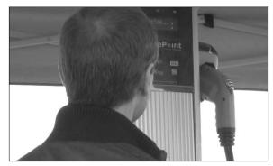
Step three: Go to charging station and swipe a special card that will allow you to take the J 1772 charging plug out of its holder
