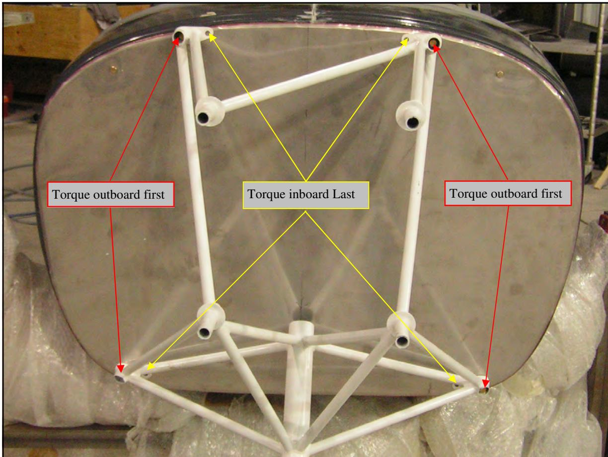
41. Torque the inboard bolts to 10ftlbs, shown in yellow in the picture above.
