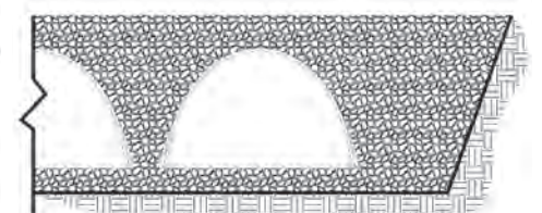
Perimeter Fully Backfilled
