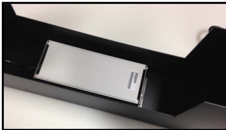
GUV C CLASSIC PLUS – Electronics are under the cover. The displays can be seen through the cover. To reset or silence the alarms, following the instructions on the front label. Basically, push button to scroll through options, once at the appropriate option, hold button to reset.
