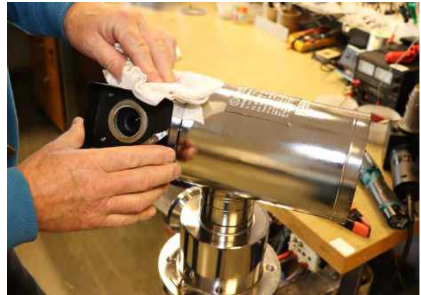
EX286W from 2007 upgraded to Ethernet-over-Coax
