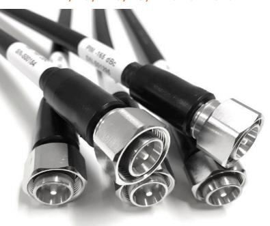
ConductRF PJA43 series of Low PIM RF Jumpers are a 100% tested to ensure minimum performance level with Typical PIM lower than -160dBc PIM. PIM Data is marked on each cable. In addition, we also fully test Loss and VSWR to ensure each assembly achieve better than its specified performance. Our range includes common standards Din7/16, 4.3/10, 4.1/9.5 & Type-N in a wide array of configurations.
