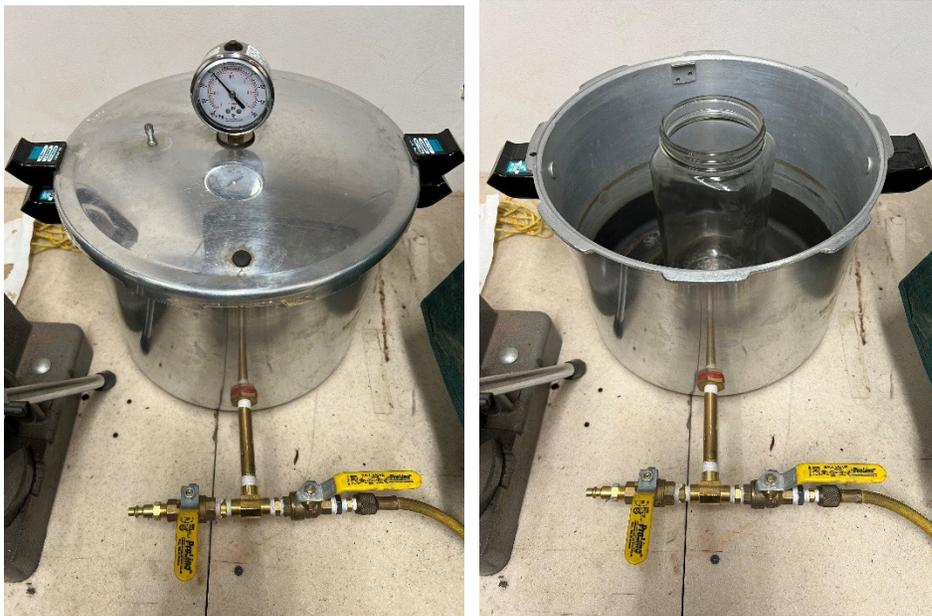
You see with the complete kits, they come with a clear acrylic top about an inch thick and you can see everything inside. With my system I'm blind. So, when you turn it on you can't see the air bubbles that look like foam. It can spill out of the jar into the pot making a mess and leaving the wood exposed.
