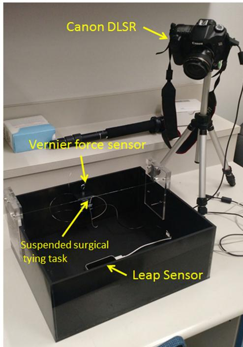
**Fig. 2** Experimental setup. Open surgery simulator with Leap Controller and Canon DSLR for real-time motion and video capture respectively
