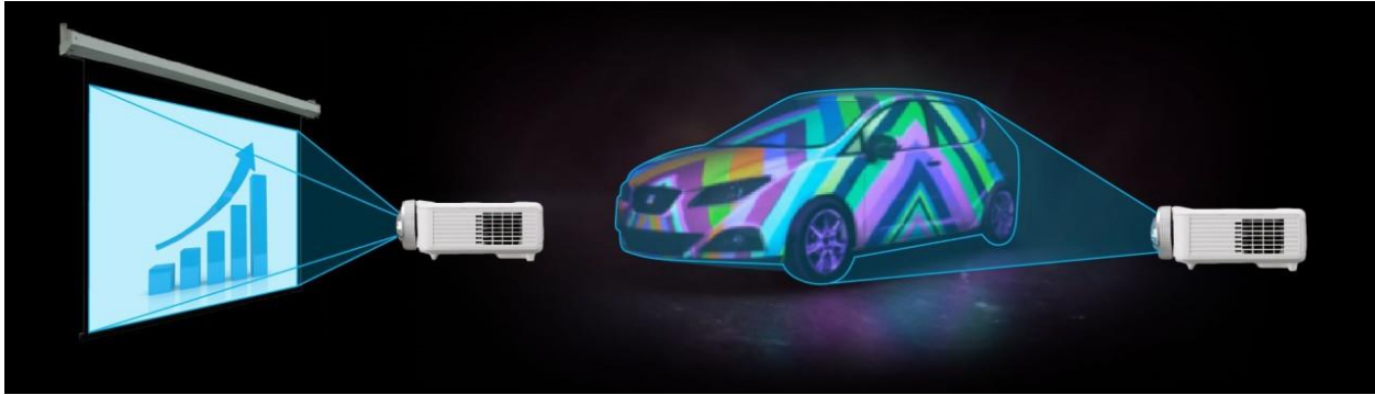
Figure 4- Display of the way a projector projects onto a non-flat surface compared to a flat surface –photo from www.Projection-mapping.org article by Brett Jones
