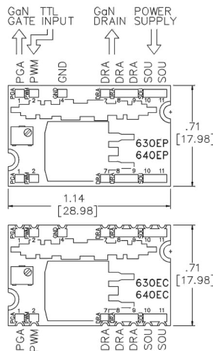
TYPE-EP typically mounts on metal surfaces, while TYPE-EC on printed circuit boards.
