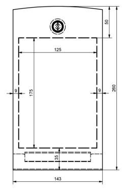
Drawing 17 - Installation range (175mm x 125mm) for fittings in the front panel
