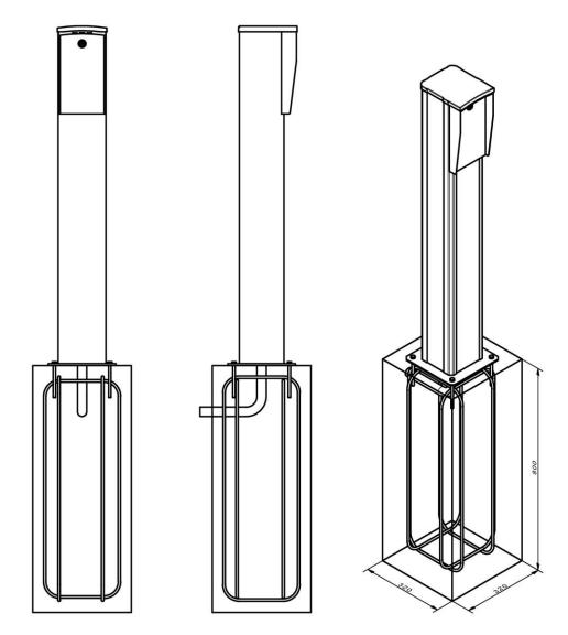
Drawing 12 - Aluminium-pillar CK with foundation incl. reinforcement and empty conduit
