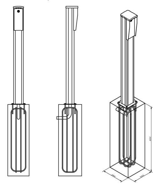
Drawing 11 - Aluminium-pillar LS and ST with foundation incl. reinforcement and empty conduit
