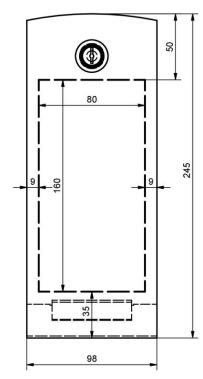
Drawing 16 - Installation range (160mm x 80mm) for fittings in the front panel
