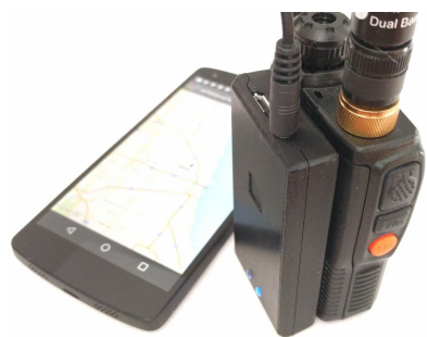
Ground Station (Non-Apple Phone, Handheld radio, Mobilinked TNC)
