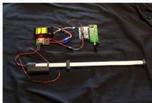
2 nd Arduino Nano and Hamshield Transceiver Interpret DTMF commands and activate Linear Actuator to push out Rover through Nose Cone end
