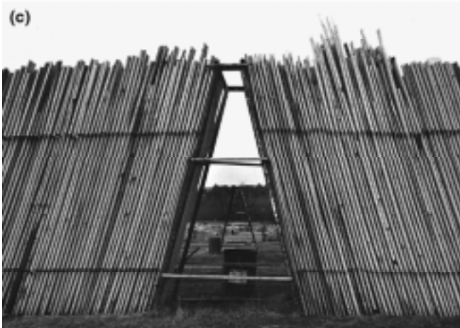
Figure 41—Alternative manual stacking arrangements that have been used in the past: (a) crib pile, (b) end racking, (c) end piling.
