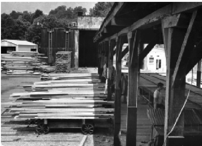
Figure 34—Hardwood lumber is graded on a conventional green chain and sorted on trucks before being stacked or sent to the automated stacker.
