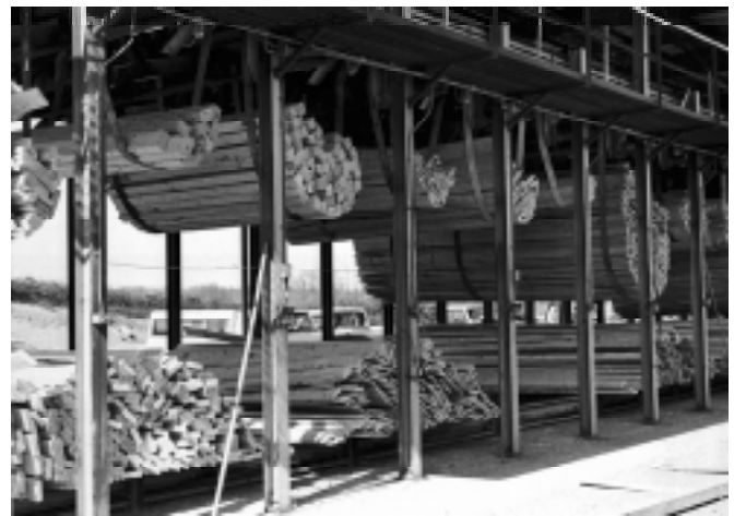
Figure 35—Sling sorter for holding lumber prior to being sent to the stacker.
