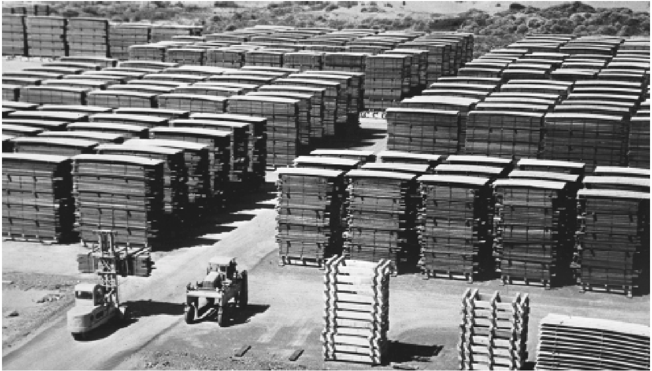
Figure 1—An air-drying yard arranged for good circulation of air around the piles of packaged lumber.
