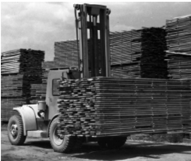
Figure 24 —In an air-drying yard, the alleys must be wide enough to enable the forklift to travel down the roadway and maneuver the package onto the pile.
