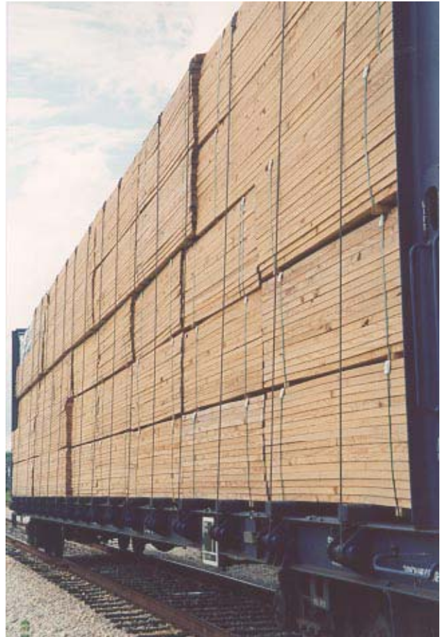
Figure 59—Flatcar loaded with lumber and held in place with cables.
