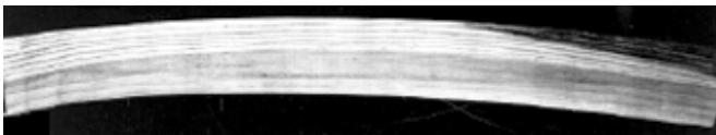
Figure 11—Crook resulted when the band of compression wood (darker strip running length of piece) shrank more longitudinally than did the lighter colored normal wood.
