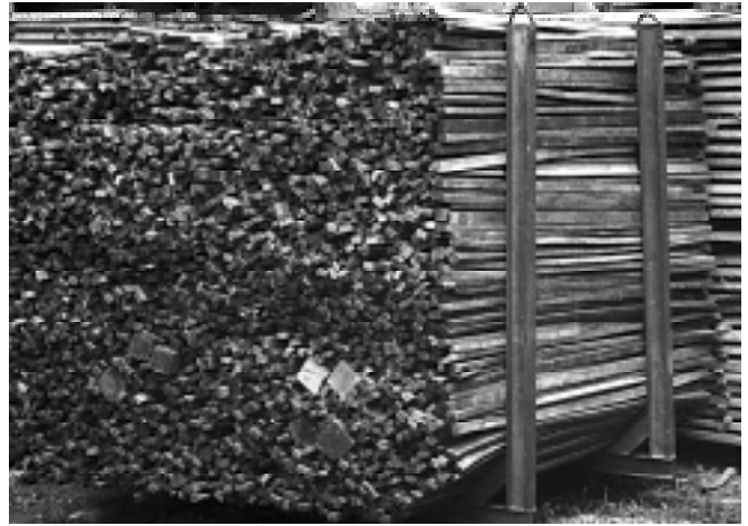
Figure 46—The handling of stickers is facilitated if they are racked for transport by forklift.
