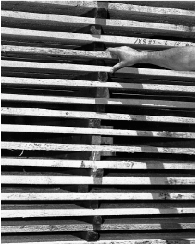
Figure 42— So that air can circulate over the board surfaces, wood stickers separate the layers or courses of lumber.
