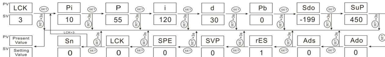
1) Pi: filtering value. Used to reduce the influence of interference.
