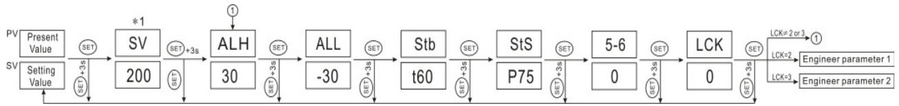
\*1: When engineer parameter SVP=0, "PV"& "SV" display as flow chart, and the setting value can be set by  $\wedge \vee$ .
