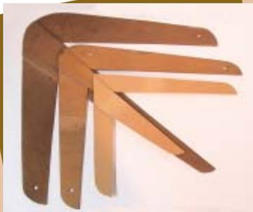
1. You need to cut a right angle square out of 1/4" bison board or custom wood. The size of the square does not matter but you can use a larger square for both large and small bowls. The three sizes illustrated range from inside square measurement of 14 1/2" down to the small one of 9 1/2".
