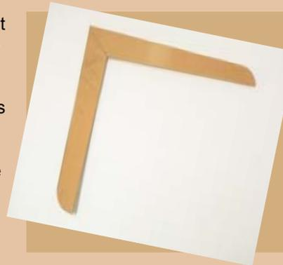
3. Then you need to bansaw out the tri-setting arm. You need to make sure that it has a straight edge. Arm ready to glue on.
