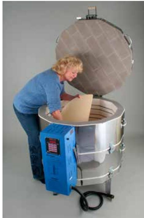
Handle kiln shelves as gently as you would a computer monitor. Avoid touching the kiln walls, thermocouple, or kiln sitter tube with a shelf.
