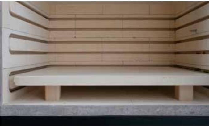
Shelves that are spaced correctly can be left inside front-loading kilns between firings. Slide ware onto them for the next firing. Shown here is a glass kiln with a single shelf that will stay inside the kiln.
