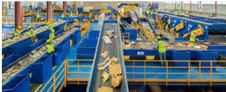
Material Recovery Facility (MRF)
